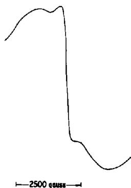
Fig. 1. Typical e.s.r. spectrum of a molybdenum trioxide doped manganese dioxide.
